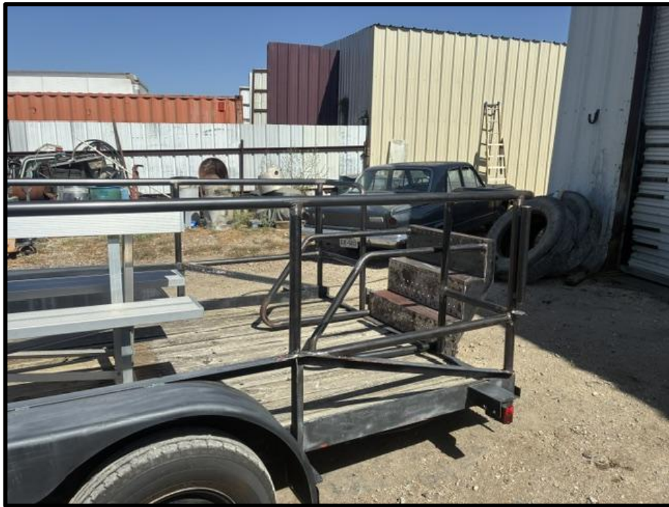
Notice the new folding steps at the rear of the trailer.
