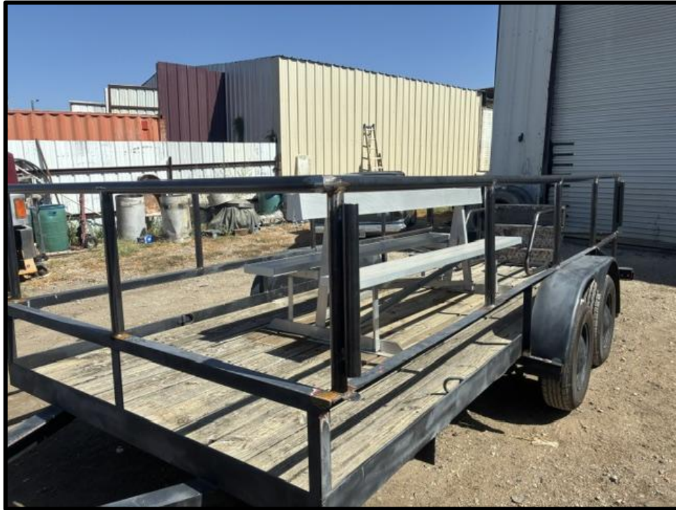
The trailer has new rails around the entire perimeter. Also, flag staff holders are on each corner.
