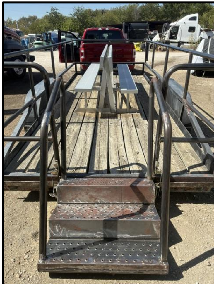
New steps with handrails will greatly assist with getting on and off the trailer.
